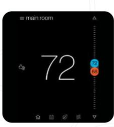
The **home screen** displays the current temperature, the current system mode, and adjustment slider, as well as icons leading to the top level screens.
