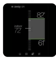
The **away screen** displays energy saving set-points. Energy saving can be invoked manually or automatically when the mobile app recognizes everyone is away.
